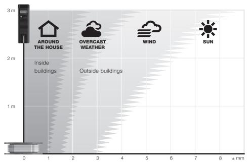
Illustration: Typical measurement reading scatter within hose radius as a function of thermal conditions and relative measuring height. For this reason no standard deviation is given.
